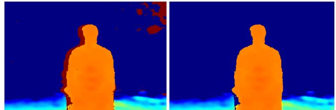
Fig. 4. The raw (left) and filtered (right) depth map.
