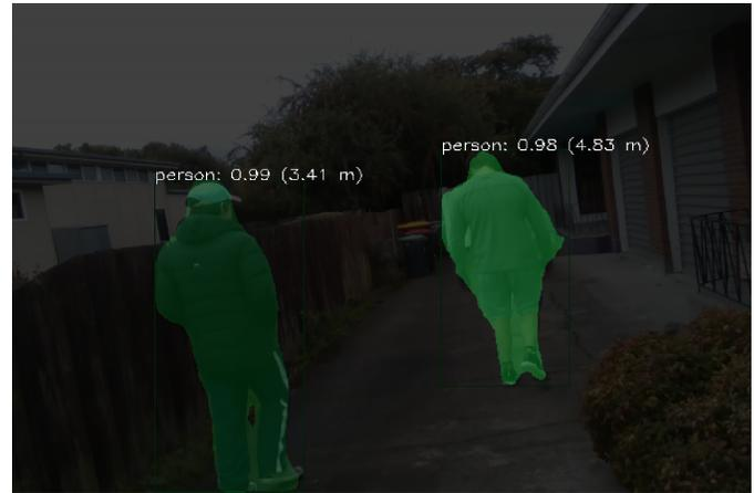
Fig. 1. An example output from our proposed method, showing multiple pedestrians identified with individual distance estimates.
