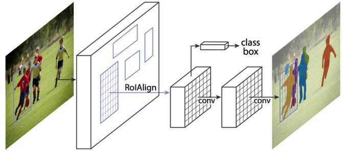
Fig. 3. A high-level architecture diagram of the Mask R-CNN framework [12].
